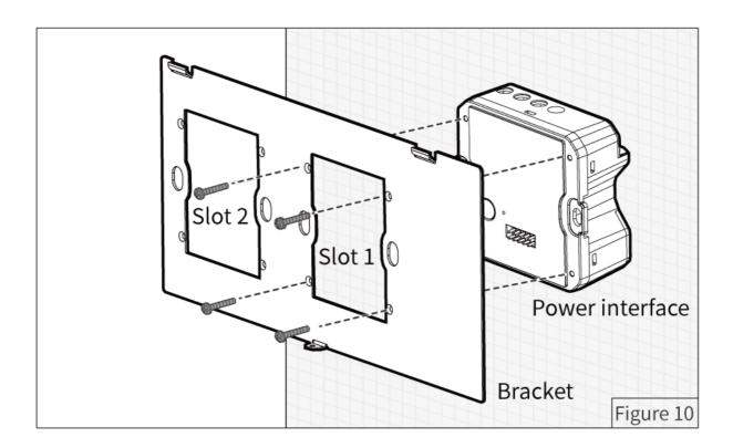
**Step 3.** Fix the power interface (already with bracket) into the wall box with screws.
