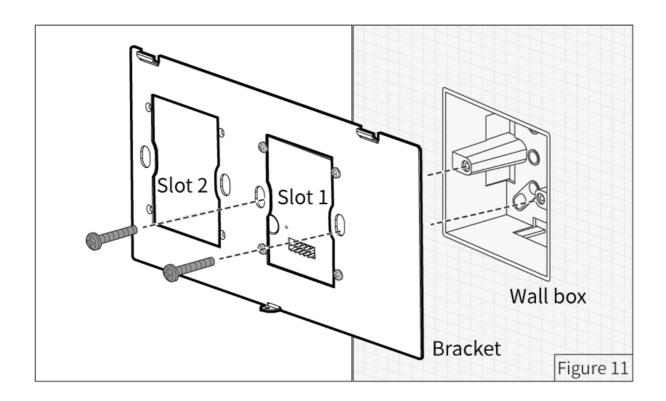
**Step 4.** Align the mounting hooks with the slots, then assemble the panel onto the bracket.
